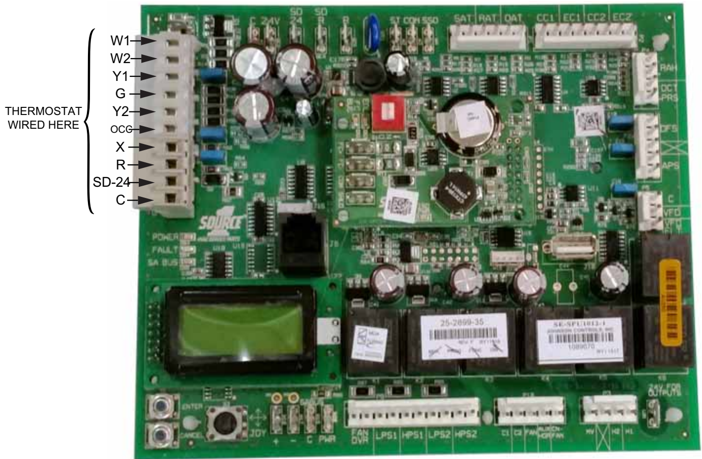
Figure 32: Unit Control Board
